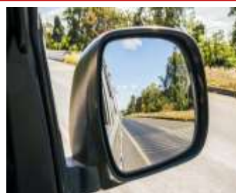
Fig. 9.7 – Use of convex mirror
